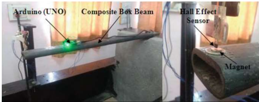
Fig. 4 Experimental setups for deflection of the beam using Hall Effect Sensor
