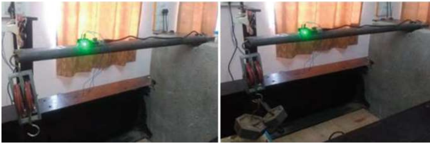
Fig. 5 Composite box beam in unloading and loading condition
