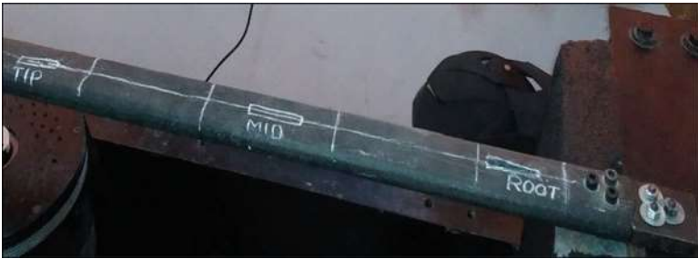
Fig. 1 Cantilever composite box beam for experimental analysis
