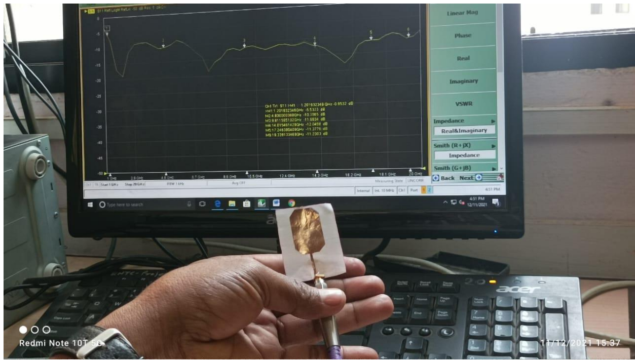
Fig. Variable Antenna for Wi-Fi, Ultra Wideband and 5G Communication
